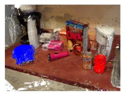
Fig. 5. 3D reconstruction of a kitchen scene with a cap highlighted in blue and a soda can in red using the labeling tool.
