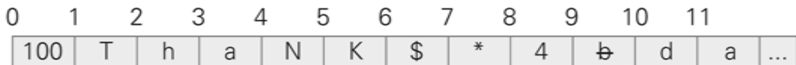
Figure 9.3. Diagram of computer memory illustrating its key properties.
