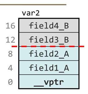
• slicing: When a derived object is converted into a base object.
