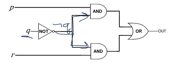
Wires can send one value to multiple gates!
