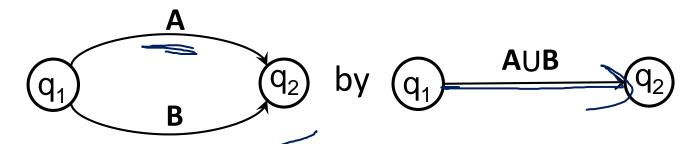
Rule 2: Eliminate non-start/final state q<sub>3</sub> by replacing all
