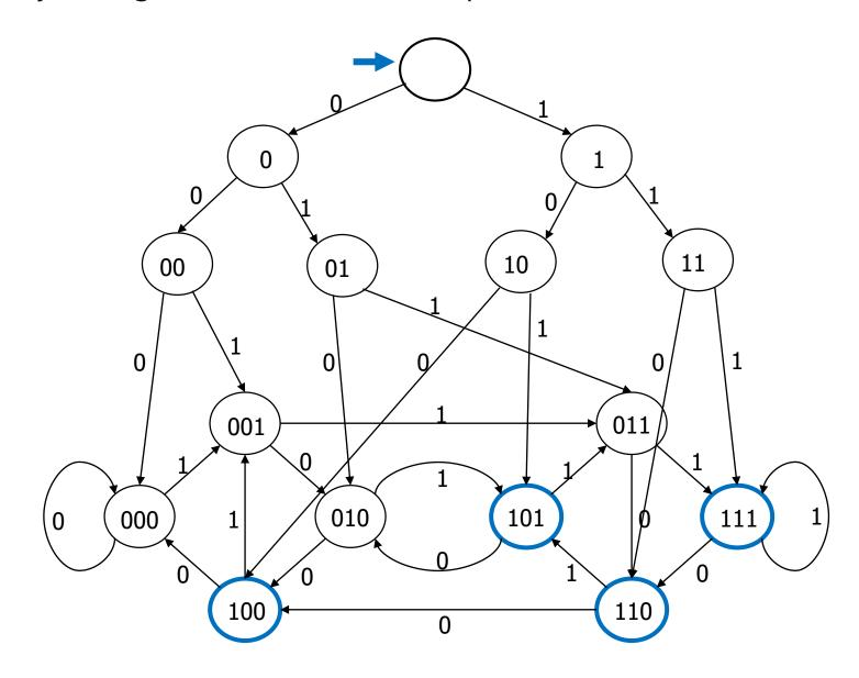
The set of binary strings with a 1 in the 3<sup>rd</sup> position from the end
