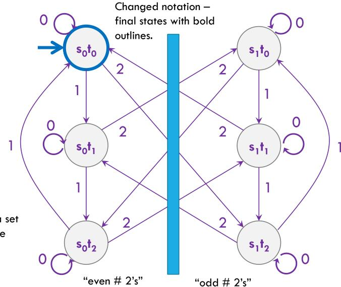
Called the "cross product" construction (because you have a set of states equal to  $Q_1 \times Q_2$  where first two DFAs had states  $Q_1, Q_2$ . A very common trick to combine DFAs.
