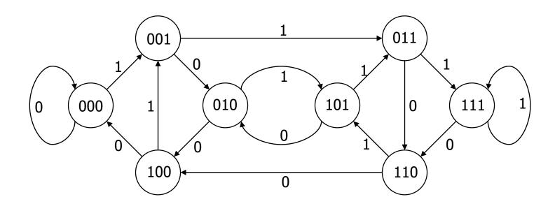
The set of binary strings with a 1 in the 3<sup>rd</sup> position from the end
