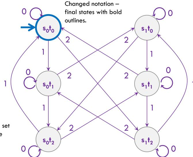
Called the "cross product" construction (because you have a set of states equal to  $Q_1 \times Q_2$  where first two DFAs had states  $Q_1, Q_2$ . A very common trick to combine DFAs.
