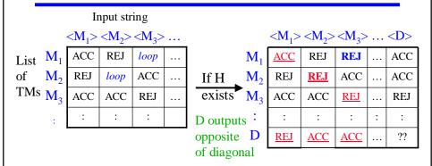
D on <M $_i>$  accepts if and only if M $_i$  on <M $_i>$  rejects. So, D on <D> will accept if and only if D on <D> rejects! A contradiction  $\Rightarrow$  H cannot exist!
