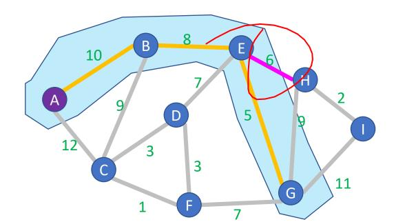
Prim's Algorithm<br/>Start with an empty tree A<br/>Pick a start nodeKeep edges in a Heap<br/> $O(E \log V)$ Repeat V - 1 times:<br/>Add the min-weight edge which connects to node<br/>in A with a node not in A
