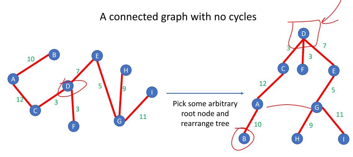
Definition: Spanning Tree A Tree  $T = (V_T, E_T)$  which connects ("spans") all the nodes in a graph G = (V, E)
