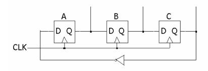
Extract the state diagram for this counter. Assume, for now, it starts in state 000. Make sure the state diagram is complete.
