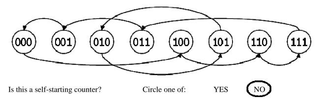
If it is not self-starting then change the equations ( $\{A.d, B.d, C.d\} = \{\-C.q, A.q, B.q\}$ ) to make the counter self-starting. Start by filling in the K-maps below from the state diagram and clearly show how to make different state transitions for the states not in the 6 state counter sequence so that the new equations will be as simple as possible.
