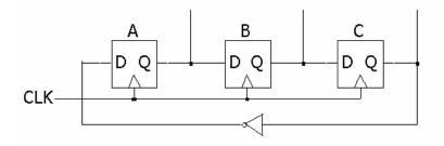
Extract the state diagram for this counter. Assume, for now, it starts in state 000. Make sure the state diagram is complete.
