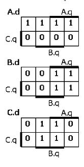
We need to change the transitions from 010 and 101 so that they fall into the 6-state counting sequence within a couple of cycles. We can do this most simply by changing the transition from 101 to 011 instead of 010. This only changes one bit in the K-maps (the bottom right cell of C.d's K-map. This makes the equations:
