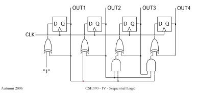
Four-bit binary synchronous up-counter Standard component with many applications positive edge-triggered FFs w/ synchronous load and clear inputs parallel load data from D, C, B, A enable inputs: must be asserted to enable counting - EN RCO: ripple-carry out used for cascading counters D C B A high when counter is in its highest state 1111 implemented using an AND gate (2) RCO goes high LOAD CLK CLR (3) High order 4-bits G are incremented (1) Low order 4-bits = 1111 ential Logic
