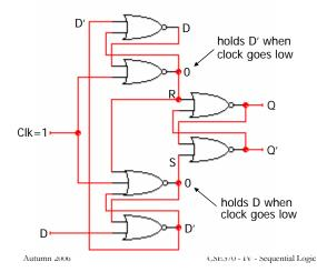
negative edge-triggered D flip-flop (D-FF)
