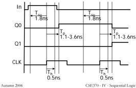
timing constraints guarantee proper operation of cascaded components
