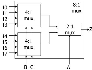
control signals B and C simultaneously choose one of I0, I1, I2, I3 and one of I4, I5, I6, I7
