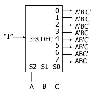
demultiplexer generates appropriate minterm based on control signals
