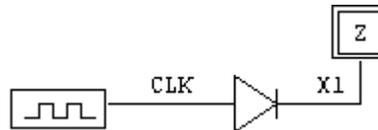
You will notice the probe is alternating between the 0 and Z states. When the input to the open-collector buffer is high, then output will be undriven and the signal will be in the high-impedance state.
