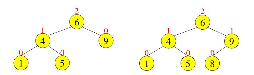
height of node = h balance factor =  $h_{left}$ - $h_{right}$ empty height = -1
