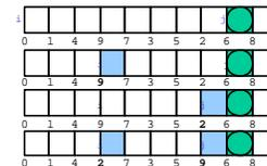
Move  $i$  to the right up to  $A[i]$  larger than pivot. Move  $j$  to the left up to  $A[j]$  smaller than pivot. Swap
