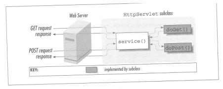
Figure 2-2. An HTTP servlet handling GET and POST requests
