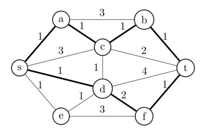
Figure 2: There are two paths (highlighted) of length 4 between s and t. The path s, d, f, t has only three edges and is the optimal solution in this example. Note that there are two s - t path (s, c, t and s, d, t) with only two edges, but they are of length 5 and are not shortest paths.
