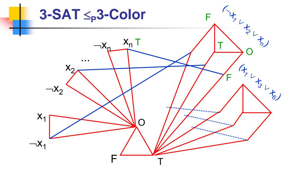
Any 3-coloring of the graph has T at the other end of the blue edge connected to the F
