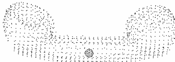
(a) Initialization with balloon entirely within the 3D point cloud.
