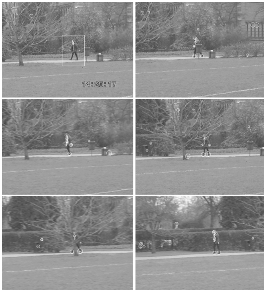
Figure 11. Results from the recognition experiment on the Vicky sequence. The model was generated from the top-left image (taken from vicky1) cropped to the rectangle. The superimposed circles show the features in each frame (of vicky2) which match with the object model.
