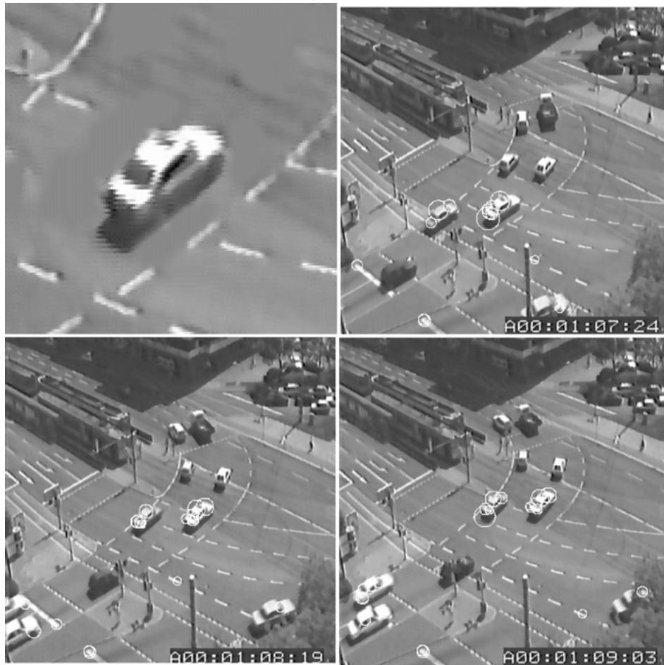
Figure 10. Results from the recognition experiment on the DT sequence. The top-left shows the (enlarged) image of the car from which the object model was built. The superimposed circles show the features in each frame which match with the object model.
