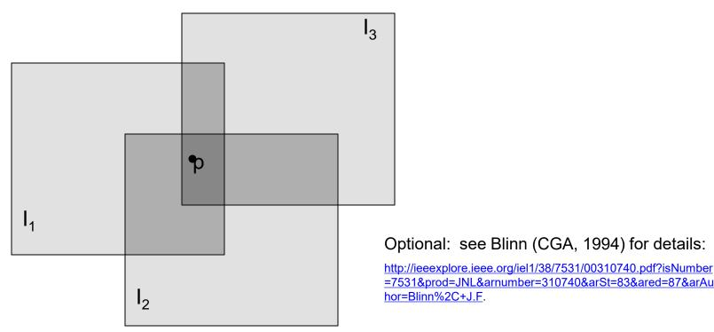
Encoding blend weights:  $I(x,y) = (\alpha R, \alpha G, \alpha B, \alpha)$
