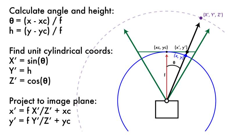
(xc,yc) = center of projection and f = focal length of camera
