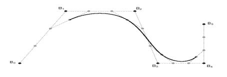
These are called **B-splines**. The starting set of points are called **de Boor points**.
