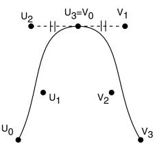
For the next two curves, the control points  $U_0$ ,  $U_1$ ,  $U_3$ ,  $V_2$ , and  $V_3$  are fixed as shown, and you must specify the locations of and label the remaining control points to establish the requested continuities. You must also sketch the resulting spline curve.
