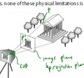
The image is rendered onto an image plane (usually in front of the camera).
