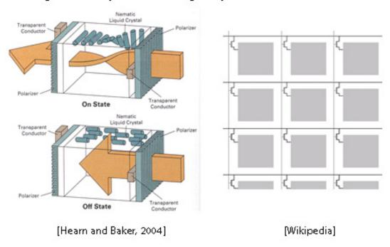
Laptops typically use **liquid crystal displays** (LCD's).
