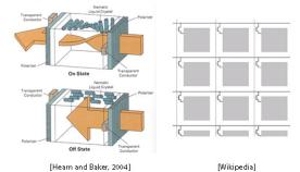
Laptops typically use liquid crystal displays (LCD's).
