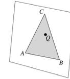
We call  $\alpha$ ,  $\beta$ , and  $\gamma$  the **barycentric coordinates** of  $Q$  with respect to  $A$ ,  $B$ , and  $C$ .
