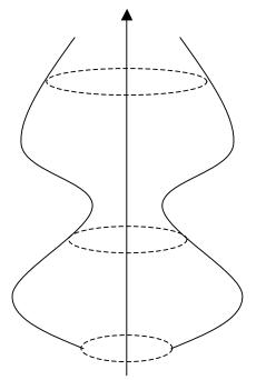
Idea: rotate a 2D profile curve around an axis.
