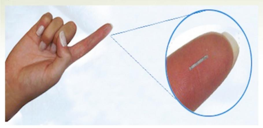
**Diabetics** rejoice: a new rice-sized, implantable glucose sensor could eliminate the need to use conventional finger-prick monitors. The solar-powered device, dubbed **Glucowizzard**, is implanted under a patient's skin, where it monitors glucose levels continuously until it needs to be replaced approximately a year later.
