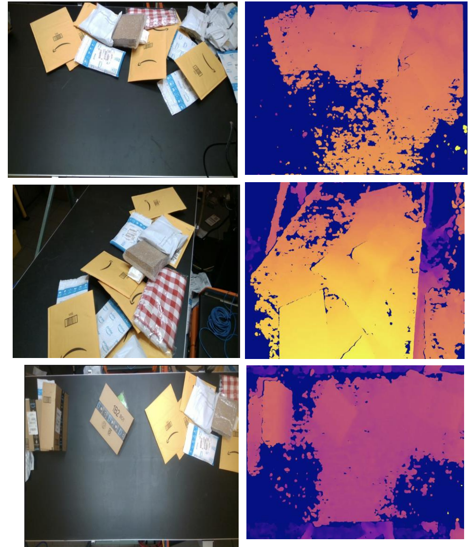
120 sets of real dataset - RGB images from 3 viewpoints and ground truth depth maps obtained from sensors T = 0, t = 1, t = 2, \dots, t = 119
