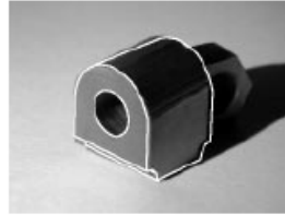
Figure 18: The pose computed from six point correspondence using the algorithm described in Section 5.2.
