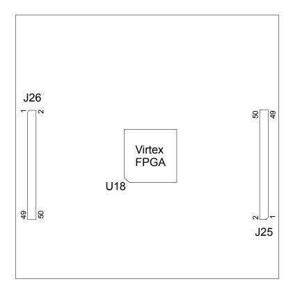
The connections between the FPGA and the expansion headers are listed below. The FPGA pins which connect to the left and right expansion headers are also connected to the left and right banks of SRAM, respectively. The SRAM bank chip-enable should be raised to disable the SRAMs on that side if the associated expansion header is being used for external I/O.
