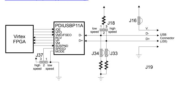
The USB port is set to high (12 Mbps) or low speed (1.5 Mbps) by shunts on jumpers J18 and J37. A 15K load can be placed on the D+ and D- USB signals by placing shunts across jumpers J33 and J34. If the USB peripheral connected to the port needs to draw power from the XSV Board, then a shunt should be placed on jumper J16.
