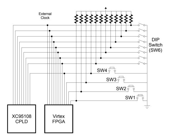
The table below lists the connections from the FPGA and CPLD to the switches. The DIP switches also share the same pins as the uppermost eight bits of the Flash RAM address bus. If the Flash RAM is programmed with several FPGA bitstreams, then the DIP switch can be used to select a particular bitstreams which will be loaded into the FPGA by the CPLD on power-up.
