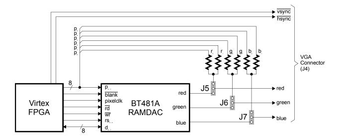
When the FPGA is directly generating VGA signals, the lower six bits of the P bus provide two-bits of red, green, and blue color information to a simple resistor-ladder DAC. The outputs of the DAC are sent to a VGA monitor along with the horizontal and vertical sync pulses (/HSYNC, /VSYNC) from the FPGA.
