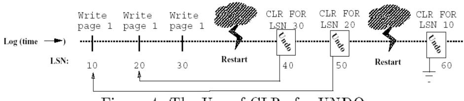
Figure 4: The Use of CLRs for UNDO
