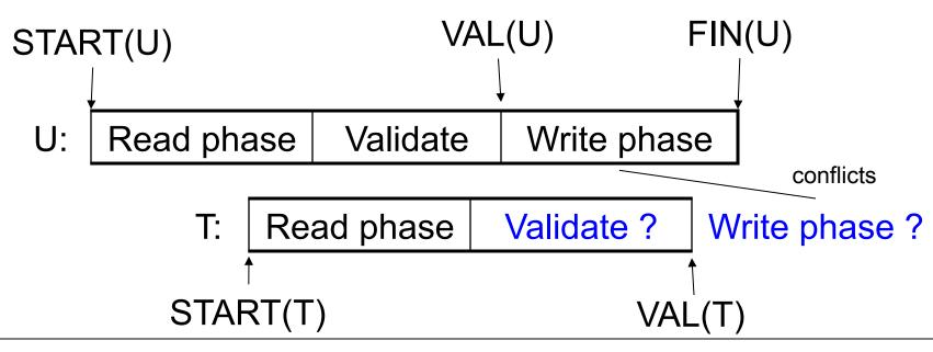
IF WS(T) ∩ WS(U) and FIN(U) > VAL(T)(U has validated and U has not finished before T validates)Then ROLLBACK(T)
