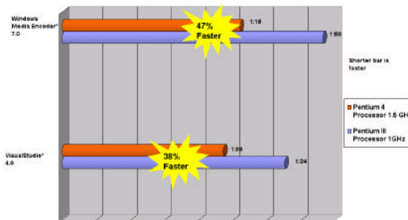
Figure 9. The Pentium 4 processor performs faster video editing, encoding on existing applications. Pentium 4 processor is 47% faster than Pentium III processor in Windows Media Encoder 7.0, and 38% faster in Ulead VisualStudio 4.0. Test configurations for video editing and encoding are listed in Section 6.
