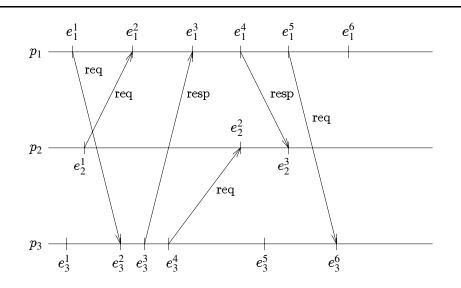
Figure 1. Space-Time Diagram Representation of a Distributed Computation
