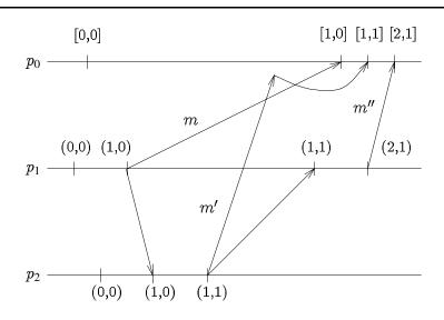
Figure 8. Causal Delivery Using Vector Clocks
