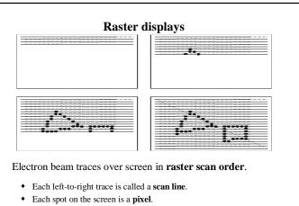
• When the beam is turned off to sweep back, that is a **retrace**, or a **blanking interval**.
