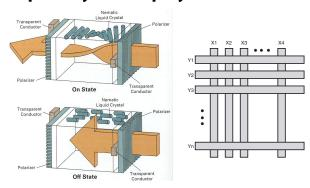
Laptops typically use liquid crystal displays (LCD's).
