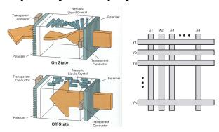
Laptops typically use liquid crystal displays (LCD's).
