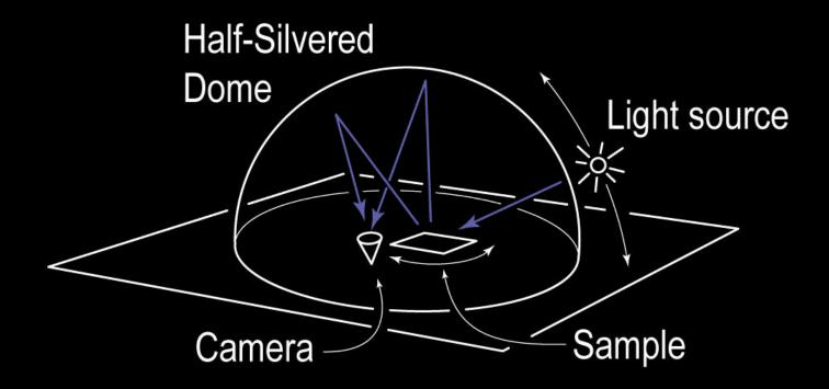
3 DOF: 2 detector, 1 source (+1 sample) Exitant directions fixed by optics; incident directions chosen
