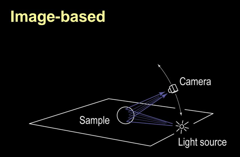
3 DOF: 2 image, 1 camera Samples arranged on 2D sheets in 3D parameter space
