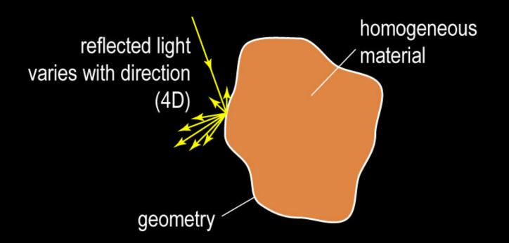
Single scattering: -1D; surface scattering: -1D Homogeneous material: -2D
