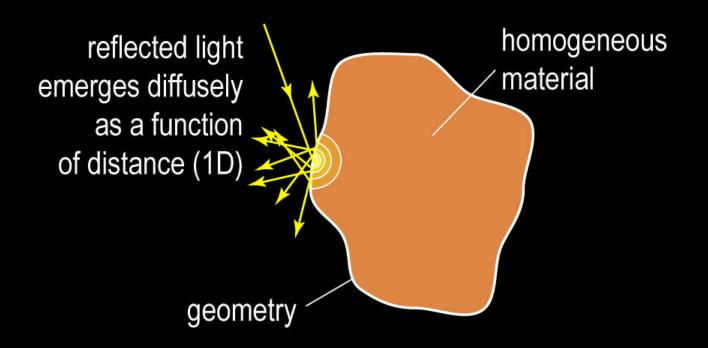
Homogeneous material: -2D Diffuse reflection: -4D; isotropic material: -1D
