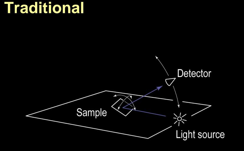
3 DOF: 2 sample, 1 detector Samples arranged on any desired grid
