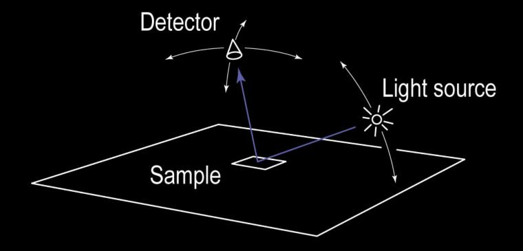
3 DOF: 2 detector, 1 source Samples arranged on any desired grid
