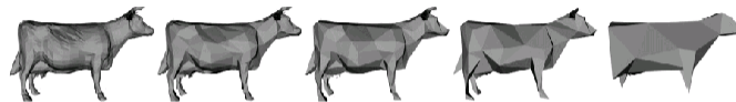
Figure 4: A sequence of approximations generated using our algorithm. The original model on the left has 5,804 faces. The approximations to the right have 994, 532, 248, and 64 faces respectively. Note that features such as horns and hooves continue to exist through many simplifications. Only at extremely low levels of detail do they begin to disappear.
