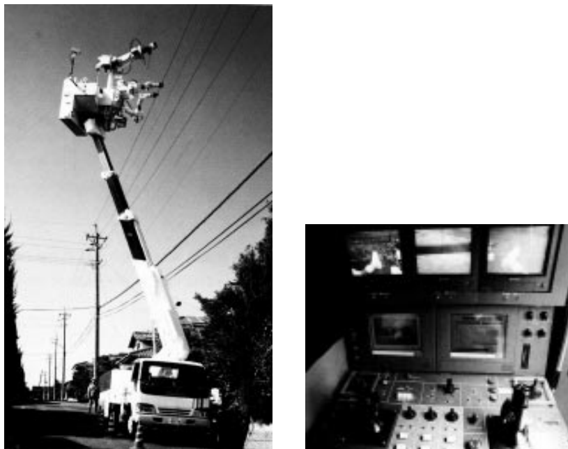
Figure 15.9: The “Hot-Line Telerobot System” from Kyushu ELeCtric Power Co. A teleoperated robot repairs a high-voltage power line (left). The operator’s interface to the system (right). (Courtesy of Blake Hannaford with permission of MIT Press. Reprinted from K. Goldberg, The Robot in the Garden , Cambridge, MA: The MIT Press, 2000.)
