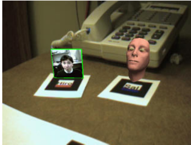
Figure 15.6: An application of augmented reality techniques to teleconferencing (courtesy of the University of Washington HIT Lab).
