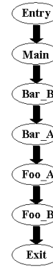
Figure 2: First Use Call Graph: The first use call graph is generated using the static first use estimation or the profile. It is then used to determine the order in which the files transfer for remote execution.
