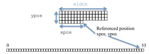
This time, we will write a simple, value returning function that converts from the 2-D view we'd like to use with the photo to the 1-D view that the pixels[] array needs.
