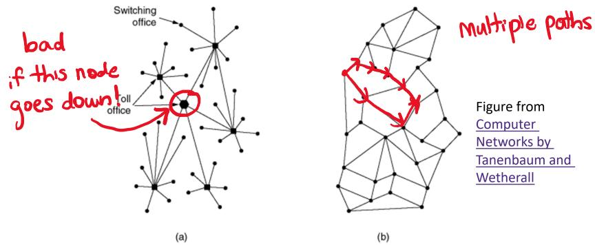
Figure 1-25. (a) Structure of the telephone system. (b) Baran's proposed distributed switching system.
