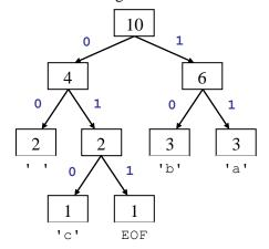
The code for each character can be determined by traversing the tree. To reach ' ' we go left twice from the root, so the code for ' is 00. The code for 'c' is 010, the code for EOF is 011, the code for 'b' is 10 and the code for 'a' is 11. By traversing the tree, we can produce a map from characters to their binary representations. For this tree, it would be:
