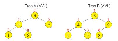
height of node = h balance factor = h<sub>left</sub>-h<sub>right</sub> empty height = -1
