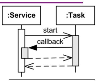
A synchronous callback. Time increases downward. Solid lines: calls Dotted lines: returns
