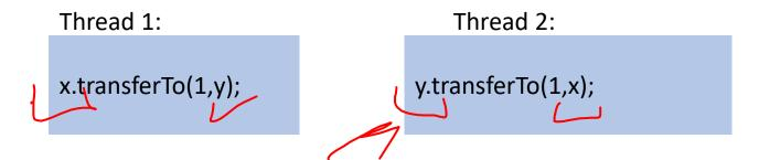
acquire lock for account x b/c transferTo is synchronized acquire lock for account y b/c deposit is synchronized release lock for account y after depost release lock for account x at end of transferTo
