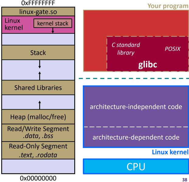
**OxFFFFFFF** linux-gate.so Process is executing your Linux kernel stack program code kernel Stack SP= **Shared Libraries** Heap (malloc/free) Read/Write Segment .data, .bss Read-Only Segment **||P □** .text, .rodata
